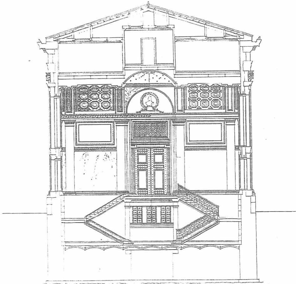
CROSS SECTION THRO' ENTRANCE HALL LIBRARY, NEW YORK UNIVERSITY, UNIVERSITY HEIGHTS, NEW YORK CITY * MCKIM, MEAD AND WHITE ARCHITECTS * 160 FIFTH AVENUE, NEW YORK CITY * * SCALE ONE INCH EQUALS FOUR FEET *
